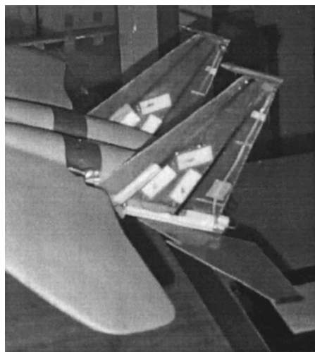
Fig. 8 Instrumented vertical tails mounted on the scale model.
