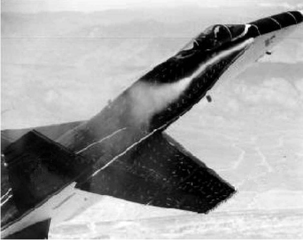
Fig. 1 Typical buffet in a twin-tail aircraft.
