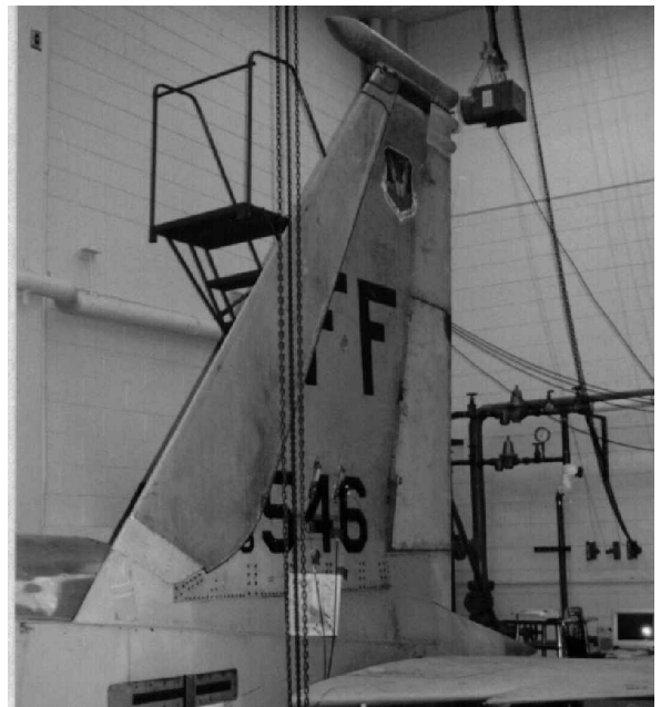
Fig. 2 Laboratory vertical tail subassembly.
